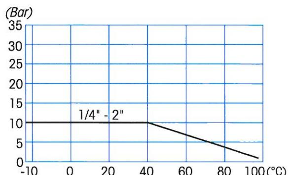
For Specifications about the Pressure-temperature Diagram and installation instructions, see page 410
